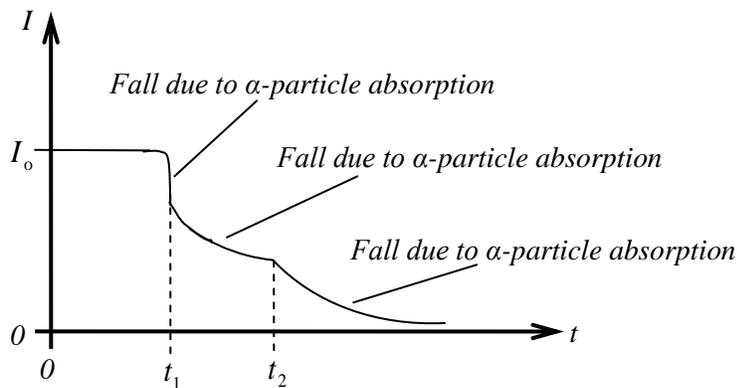
Alpha, beta and gamma radiations all pass through a very thin sheet of paper hence no loss of intensity to a thickness,  $t_1$ .
