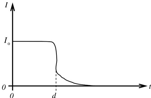
**Variation of intensity,  $I$  with thickness,  $t$  of the absorber for alpha particles.**
