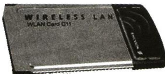
Fig.: The PCMCIA card used to connect a device to a wireless LAN
